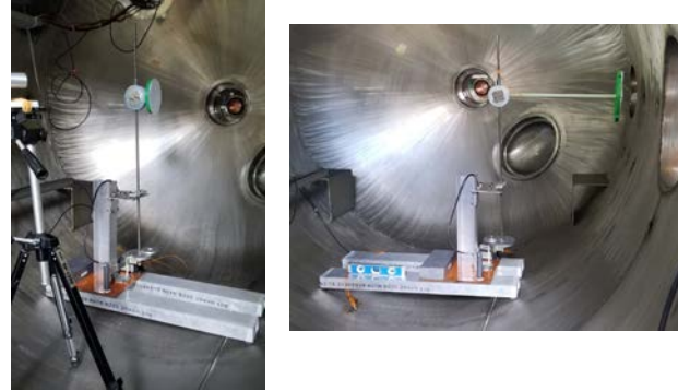
Figure 28. Left: QFP disk mounted on thrust stand roughly 0.9 m downstream of nozzle. Right: Large disk mounted on extension positioned 10 cm downstream to capture all the Neon neutral beam.
