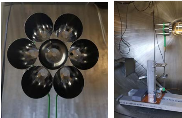
Figure 30. Right: Thrust stand setup for scoop drag force measurement. Left: image of scoop taken through neutral beam vacuum port.
