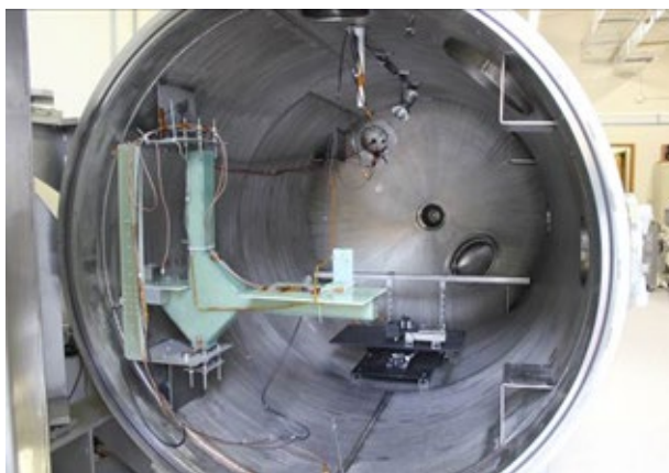
Figure 22. The 2 m diameter 4 m long MSNW large vacuum chamber with dielectric, asymmetric torsional thrust stand (green G10 garolite).
