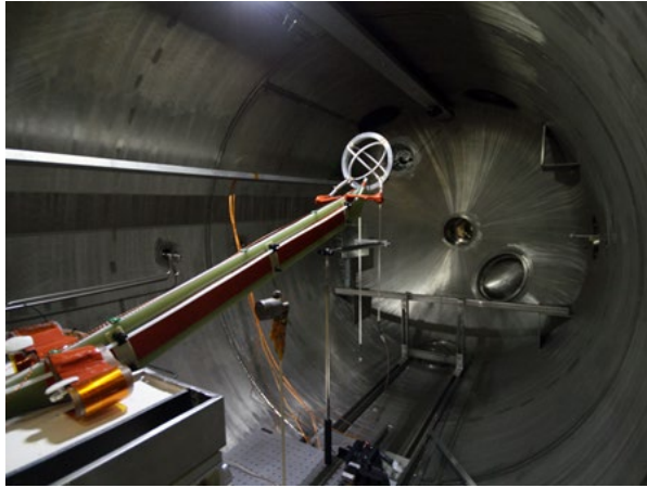
Figure 24. PMS installed in chamber. Shown are two in-chamber power supplies (potted), low-inductance stripline, G-10 mount
